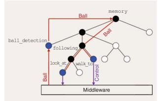
**Figure 3.** The flows of information are monitored during runtime to implement sensory–motor couplings, here for having the robot tracking the ball.
