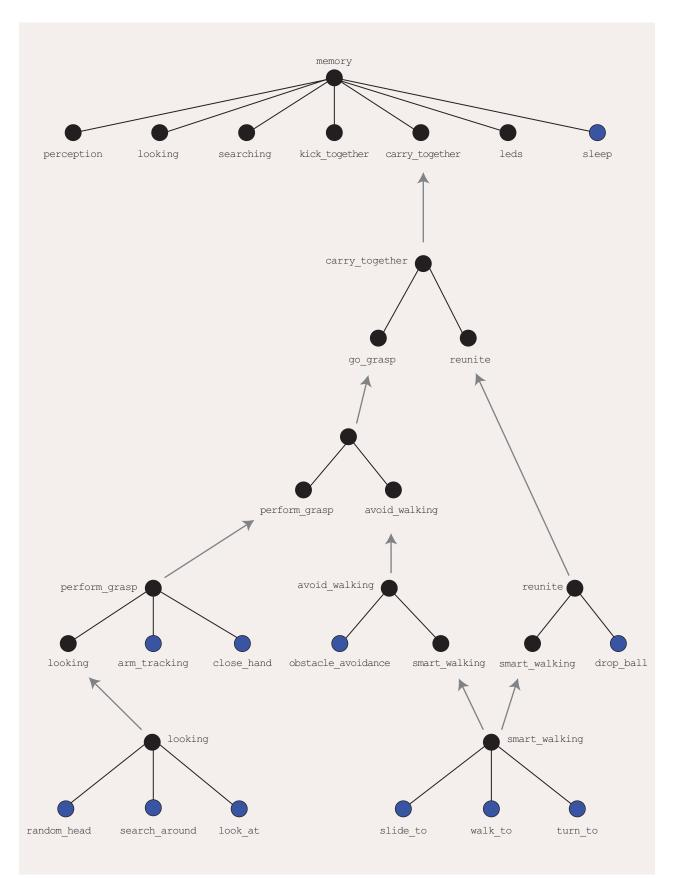
**Figure 7.** The iterative development of the carry\_together subtree of the reuniting application for Nao. In blue are leaf nodes. From bottom to top, trees of small size are created and debugged and then used as leaf nodes of trees of higher levels of abstraction. Other nodes of the full application, e.g., kick\_together, are developed using a similar approach (but are omitted here for brevity).
